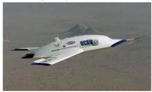
UCAV stands for Unmanned Combat Aerial Vehicle. UCAVs are unmanned aerial vehicles equipped with armaments (most commonly missiles) that have no human pilot on board, but are most times under full-time remote human control. UCAVs are usually relatively small and light, as they
